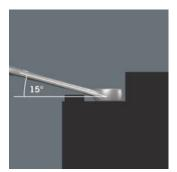
The ring side is tilted at 15° to the tool axis to prevent injury.
