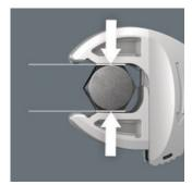
The parallel smooth jaws of the Joker 6004 allow surface pressure and can thus prevent rounding of the bolt or screw head, which can occur during power transmission via the corners.
