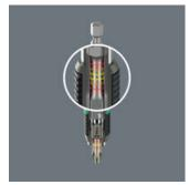
The torsion spring integrated into the unique BiTorsion holder absorbs lower levels of peak loads (Phase 1). Any overloading of this spring is effectively prevented by means of a supporting mechanism.
