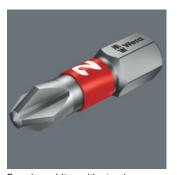
Premium bits with torsion zone into which kinetic energy is dissipated during peak loads. With softer BiTorsion zone to prevent the bit tip from twisting at high loads. This significantly increases product life. Tough design for universal use.
