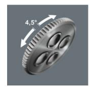
The integrated ratchet with fine toothing (80 teeth) and a return angle of 4.5° eases and accelerates screwdriving without having to reposition the tool.
