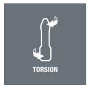
Torsion bits (T) absorb the damaging peak torque loads in the torsion zone. This prevents premature wear and enhances the service life of the bits.
