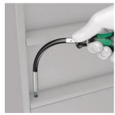
Around the corner screwdriving with the 393 S bitholding screwdriver. The flexible shaft allows to reach fixing screws in unfavourable positions. The ideal tool for srewdriving situations that are difficult to reach.
