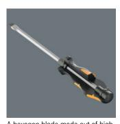
A hexagon blade made out of highquality bit material extends right through the handle - thereby ensuring full transfer of force, even when struck with a hammer. The ductile tempered material prevents the blade from splintering or breaking.
