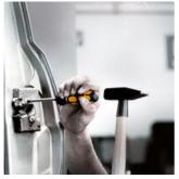
Screwdrivers are often misused as chisels. This can be dangerous. The chiseldriver is the solution when not only screwdriving is required. For fastening, chiselling and loosening seized screws. Wera chiseldriver: the screwdriver whenever the going gets tough!
