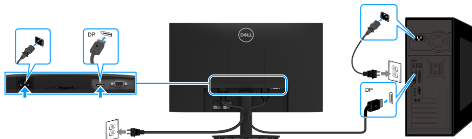
Figure 15. Connecting DP cable
