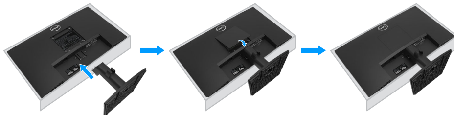
Figure 13. Attach the stand
