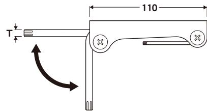
Folding multi-wrenches set comes in a steel container for easy carrying. The steel container serves as a durable handle that enables wrenches to be used at desirable inclination.
