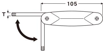
Wrenches can be adjusted in desirable inclination according to the usage purpose of quick pre-fastening and / or high torque tightening.
