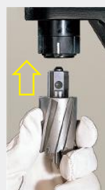
Mounting the cutter
