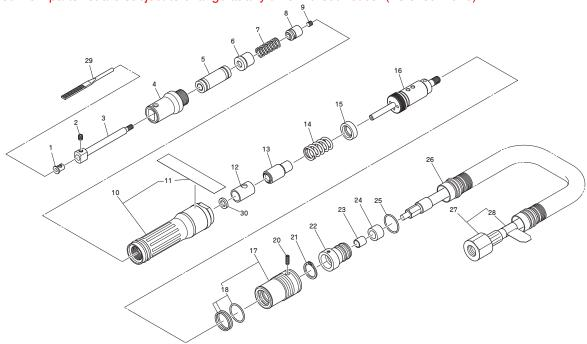
The parts numbers with ( ) are included in the Ass'y parts written above them. Numbers attached with  $\bigcirc$  are components of MAH-16.
