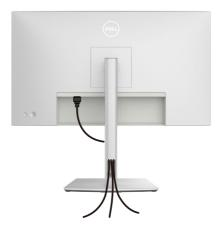
When connecting the necessary cables (for more information, see **Connecting your monitor**) route the cables through the cable-management slot.
