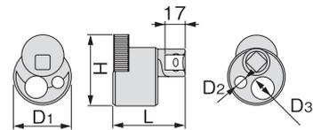
For detaching worn out bolts/nuts, 5 sizes available.
