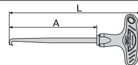
Specialized tool for attaching and detaching air valves for tires such as automobiles and motorcycles.
