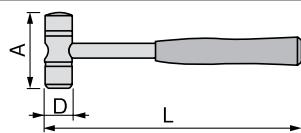
High-strength hammer with steel and urethane mallet.
