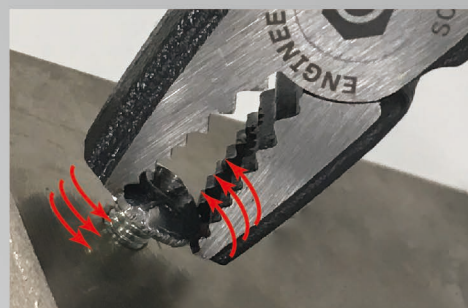
Screw Head Size ø3 - 11mm
