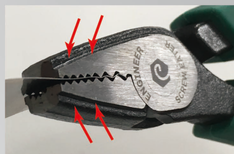
Vertical Serrations generate gripping power
